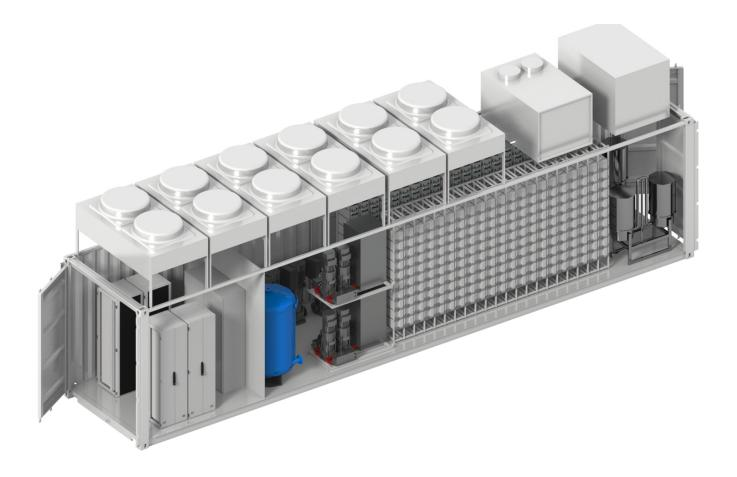
The Enapter Electrolyser AEM Multicore is packaged in a 40' container, largely pre-assembled for fast commissioning. Site works are limited to the installation of fluid lines, grid connections and the HVAC system on the container roof.
